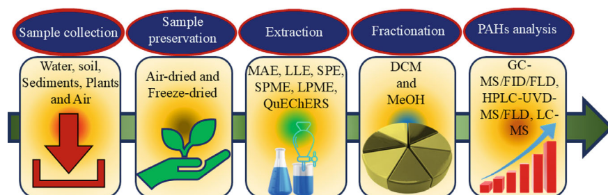
Fig. 9.2 General procedure for extraction and detection of PAHs
