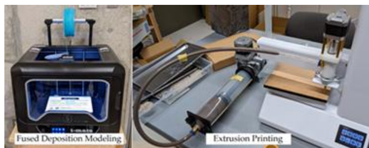
Figure 1: Extrusion printing and deposition modeling were combined to create a 3D printer
