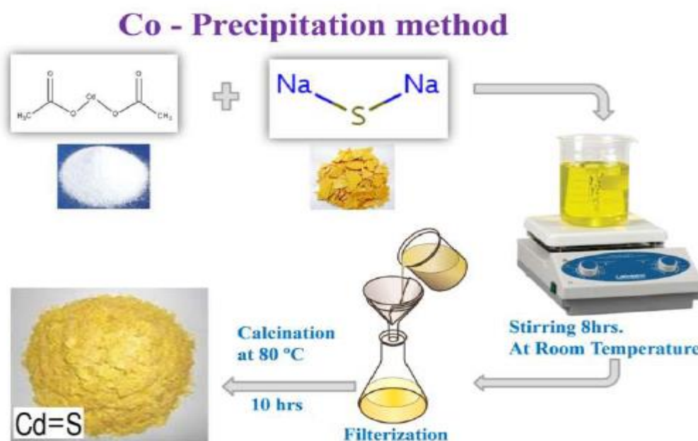
Fig. 1: A flow chart Diagram of synthesis of CdS Nanomaterial
