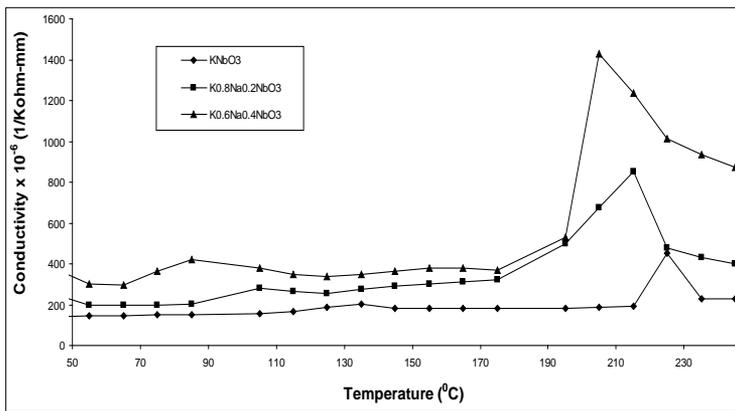
**Fig 6:** Variation of electrical conductivity with temperature for K1-X Na<sub>x</sub>NbO<sub>3</sub> system at 1 MHz
