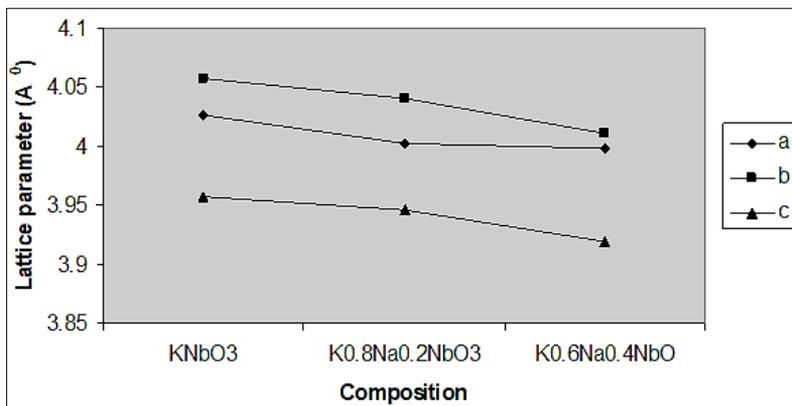
**Fig 1:** Composition dependence of lattice parameters
