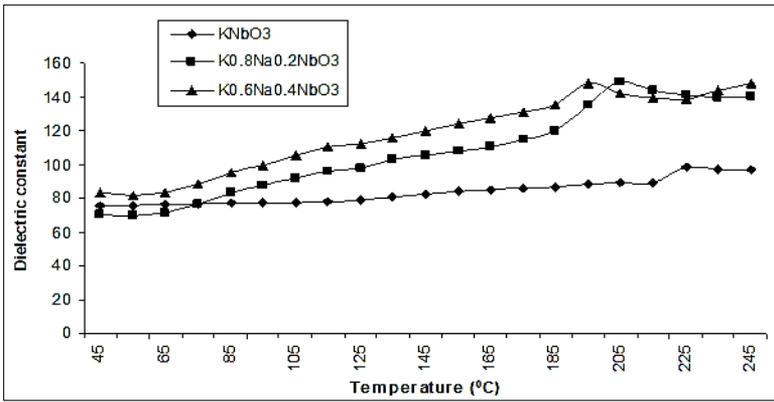
**Fig 2:** Variation of dielectric constant with temperature for  $K_{1-x}Na_xNbO_3$  at 1 MHz
