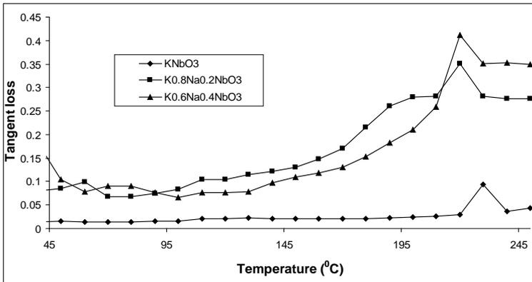
**Fig 5:** Variation of tangent loss with temperature for K1-X Na<sub>x</sub>NbO<sub>3</sub> at 100 KHz
