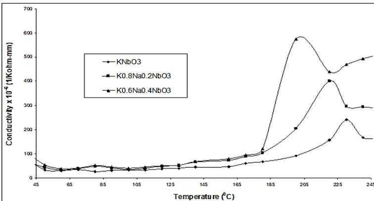
**Fig 7:** Variation of conductivity with temperature for K1-X Na<sub>x</sub>NbO<sub>3</sub> system at 100 KHz
