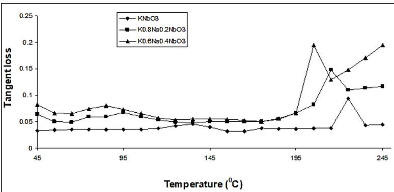
**Fig 4:** Variation of tangent loss with temperature for  $K_{1-x}Na_xNbO_3$  system at 1 MHz
