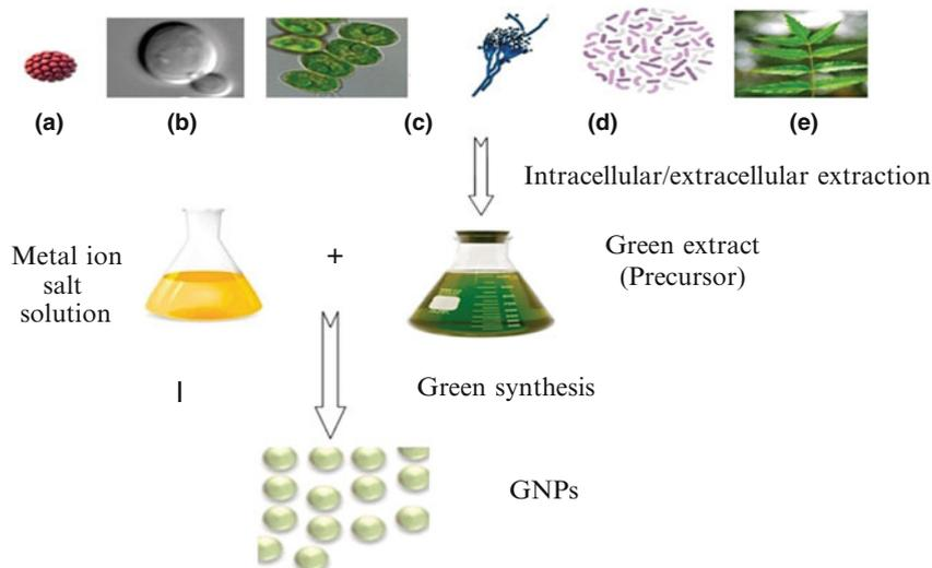
**Fig. 1** Schematic representation for preparation of green NPs. (Reprinted from original article by Dutta and Das 2021 after permission through RightsLink)
