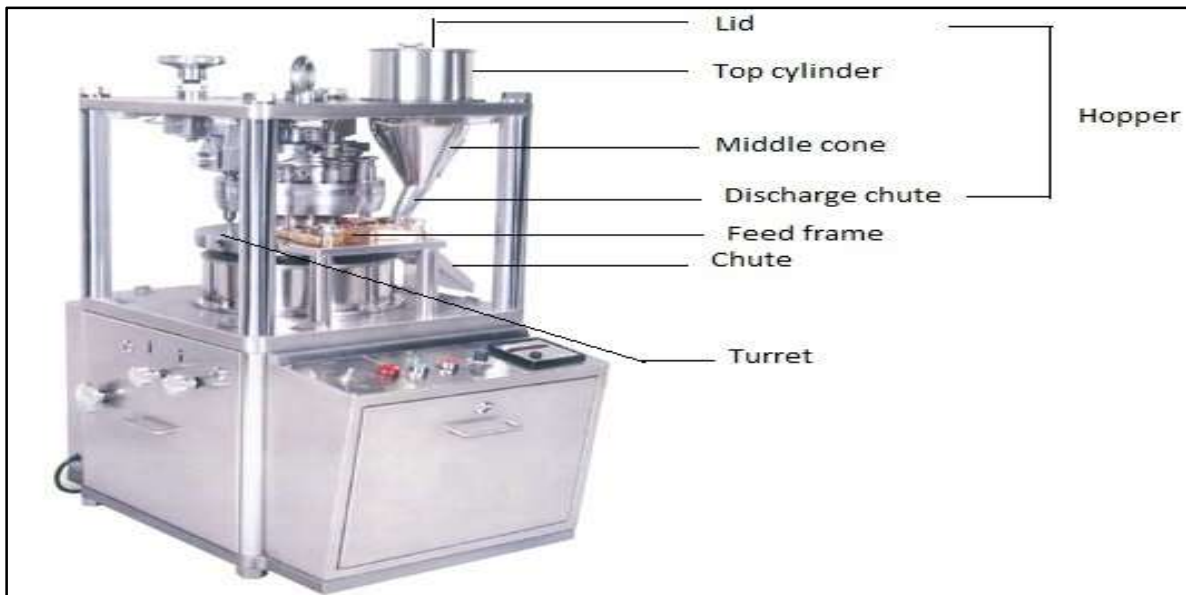
Fig. 1. Tablet Compression Machine.
