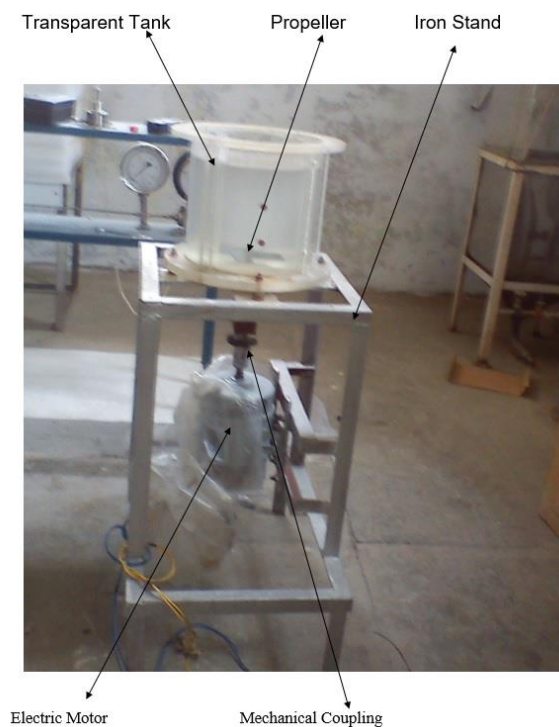
Figure 1 Experimental Setup of slurry Pot Tester
