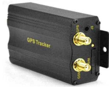
Fig. 4. An illustration of a TK103 GSM/GPRS/GPS tracker for automobiles
