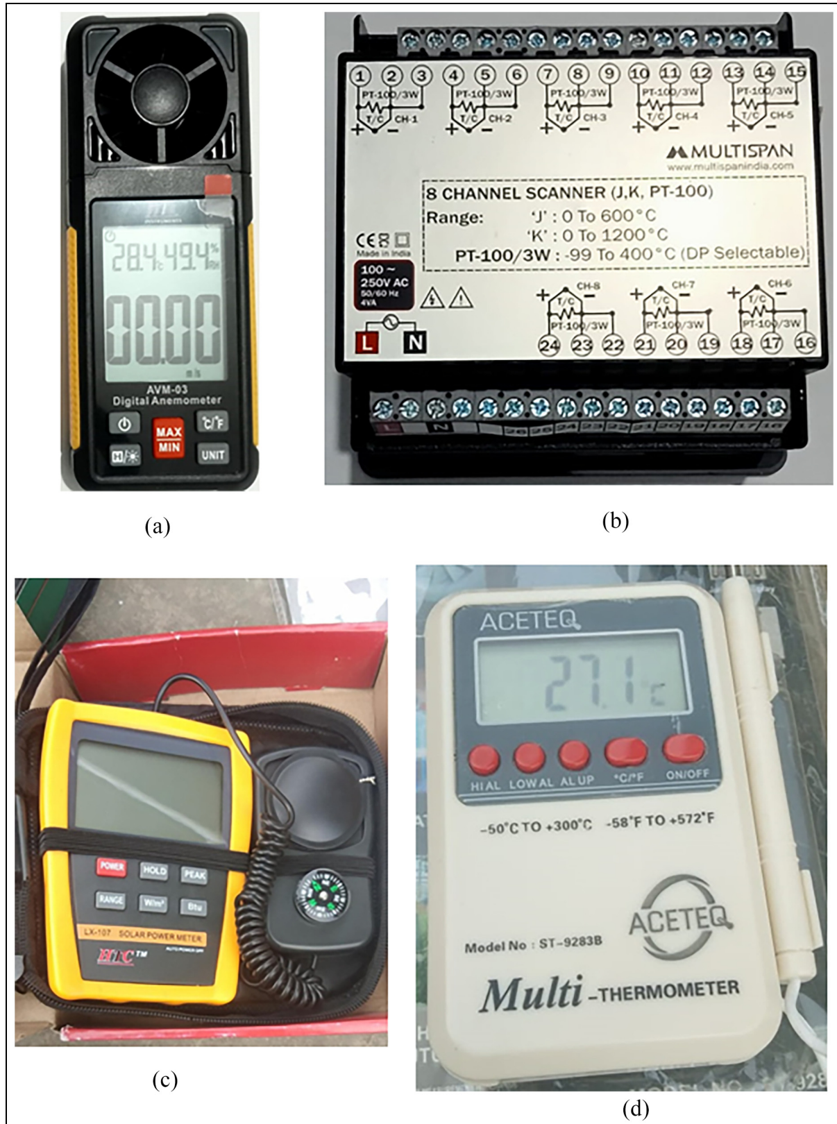
Figure 9. Instruments used in experimental work: (a) anemometer, (b) 8 channel thermocouple connector, (c) pyranometer, and (d) multi thermometer.
