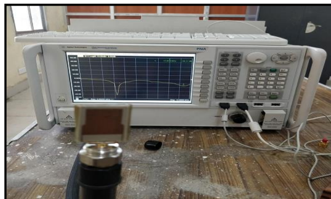
Fig.7. Measurement of the fabricated antenna using VNA
