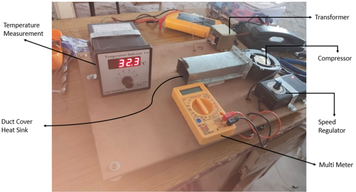
Fig. 6 Experimental setup of the heat sink cooled by atmospheric air
