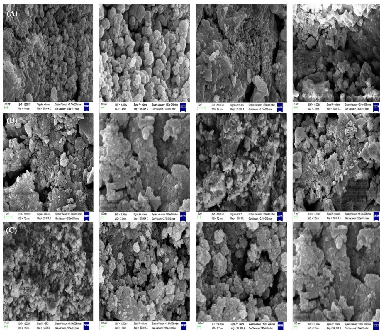
**Fig. 2** SEM images of  $\text{Pr}^{3+}$  doped CdS nanoparticles prepared by simple chemical aqueous precipitation method for (A) 0.1 mol %, (B) 0.2 mol % and (C) 0.3 mol % doping concentration of  $\text{Pr}^{3+}$  ions at room temperature
