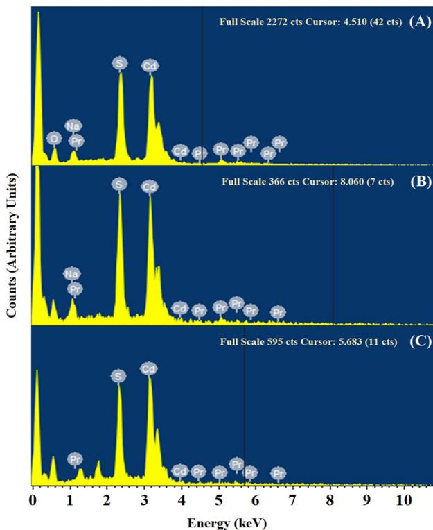
**Fig. 3** EDAX spectrum of CdS nanomaterial with (A) 0.1 mol %, (B) 0.2 mol % and (C) 0.3 mol % doping concentration of Pr<sup>3+</sup> ion
