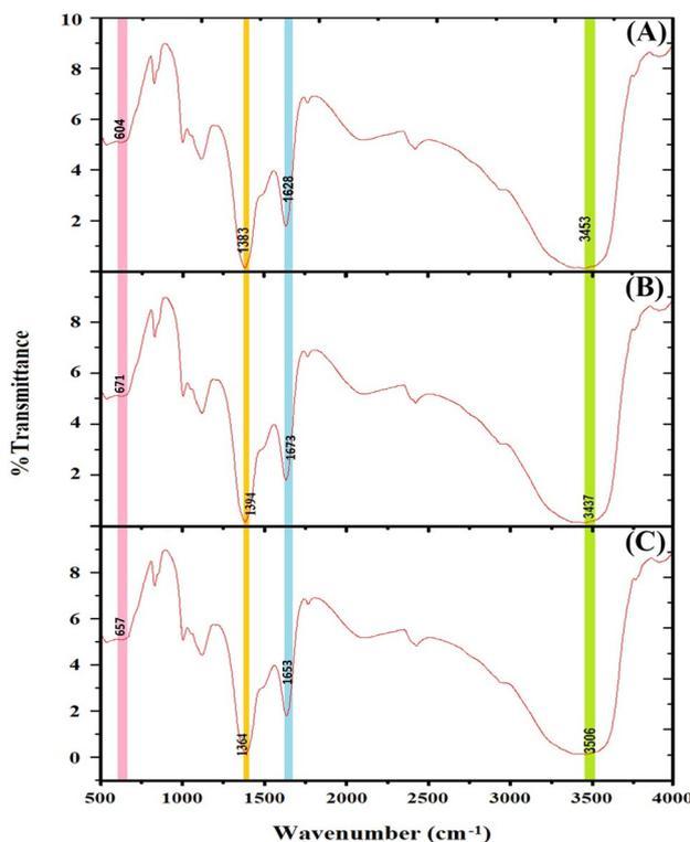
**Fig. 4** FTIR spectrum of CdS nanomaterials with (A) 0.1 mol %, (B) 0.2 mol % and (C) 0.3 mol % of Pr<sup>3+</sup> ion
