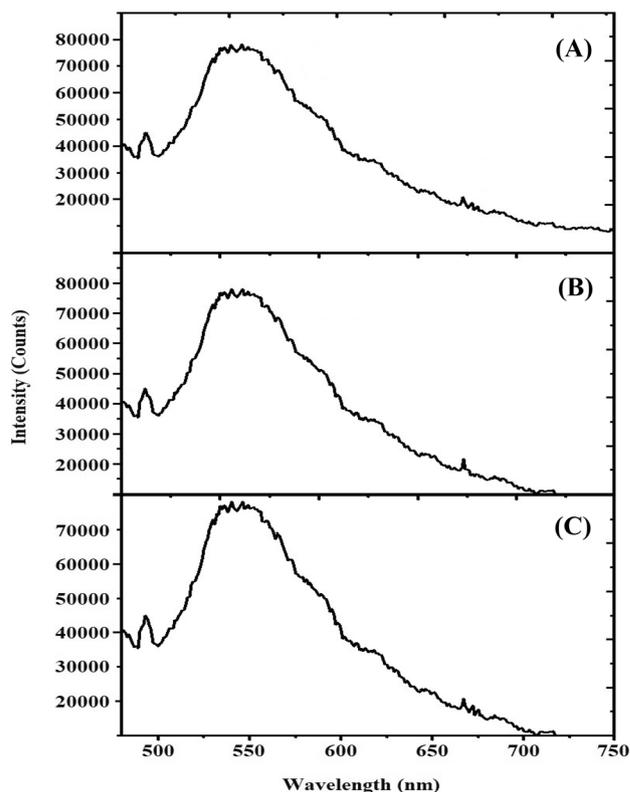
**Fig. 5** Fluorescence spectrum of CdS nanomaterial with (A) 0.1 mol %, (B) 0.2 mol % and (C) 0.3 mol % Pr<sup>3+</sup> ion
