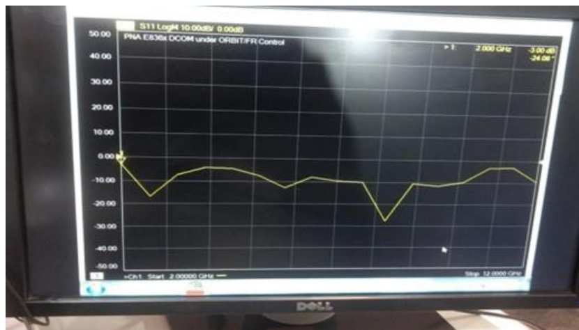
Figure 7: Measured S_{11} of the proposed notched antenna (with notch centered around 7 GHz).
