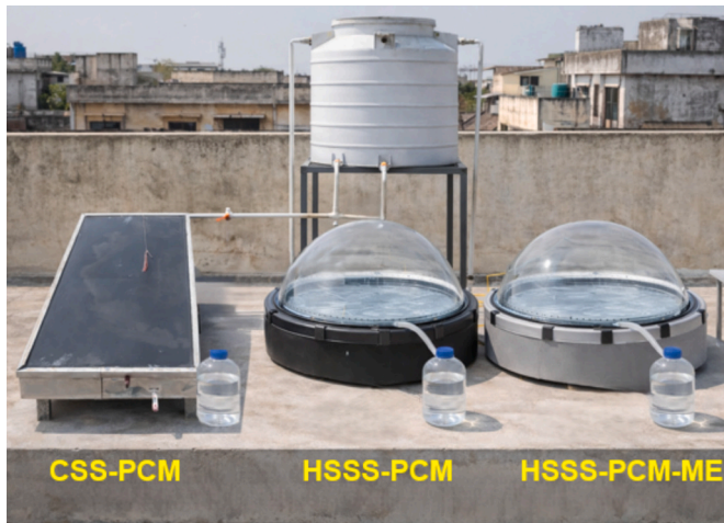
Fig. 1. Experimental setup of solar stills integrated with PCM namely Conventional single slope solar still (CSS-PCM), Hemispherical Solar still (HSSS-PCM), Hemispherical Solar still (HSSS-PCM-ME).
