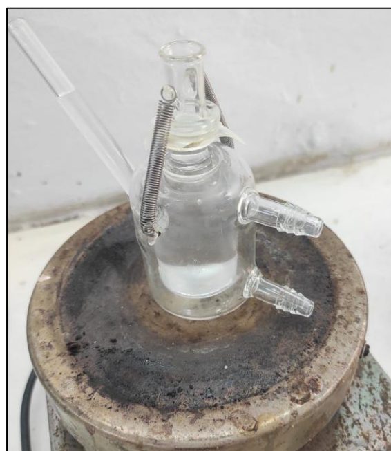
Fig. (3). In-vitro skin permeation study using franz diffusion cell. (A higher resolution / colour version of this figure is available in the electronic copy of the article).
