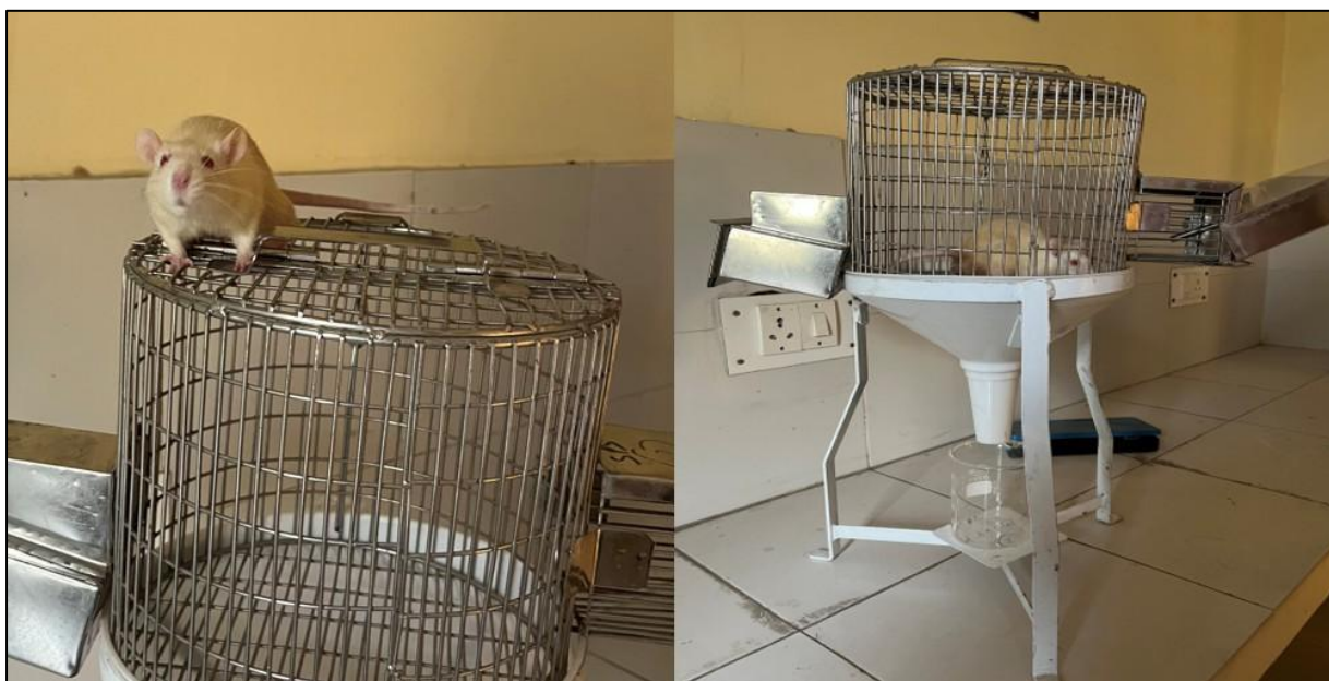
Fig. (4). Metabolic cage with an albino rat for urine collection. (A higher resolution / colour version of this figure is available in the electronic copy of the article).
